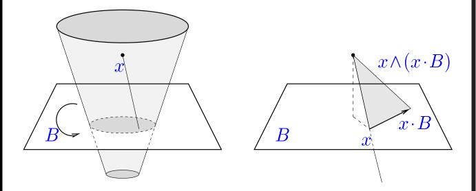
The body rotates in the B plane, at angular frequency |B|. The momentum density is  $\rho x \cdot B$ . Angular momentum density is  $x \wedge (\rho x \cdot B)$ . Integrate to get the total,  $\mathcal{I}(B)$ , expressed in the reference body. Rotate to
