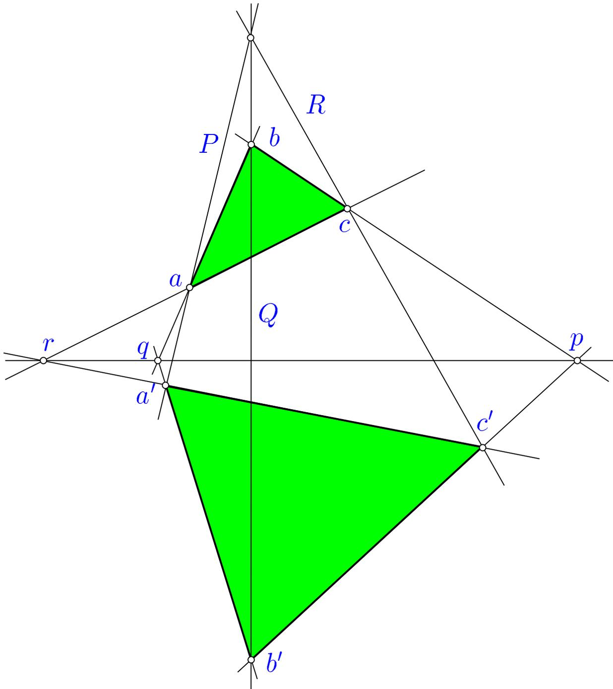
Two triangles in a plane, points  $a, b, c$  and  $a', b', c'$ . The lines  $P, Q, R$  meet at a point if and only if the points  $p, q, r$  all lie on a line. The triangles are then projectively related.
