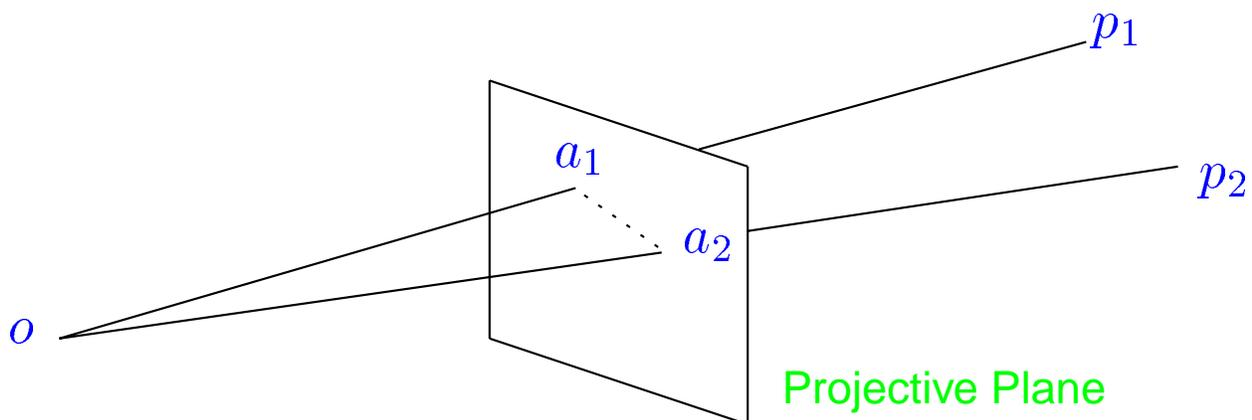
Vectors in 3-d space projected onto a 2-d plane. **Points** in the plane ( $a_1, a_2$ ) represented by **vectors** is a space of **one dimension higher**. Magnitude of the vector is unimportant —  $a$  and  $\lambda a$  represent same point. Does **not** mean there is no role for the dot product.
