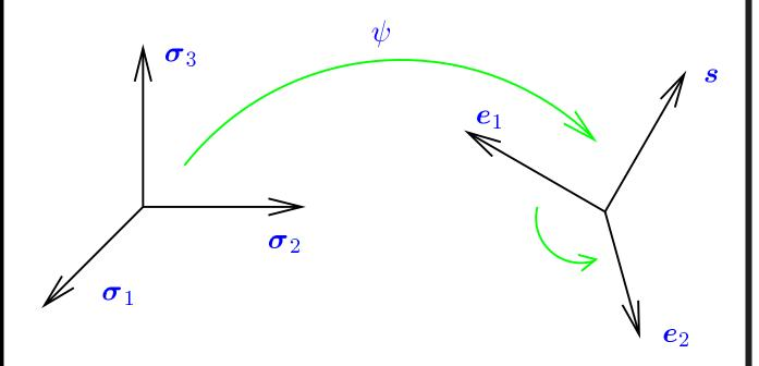
Figure 1: *The Spin Vector*. The normalised spinor  $\psi$  transforms the initial, reference frame onto the frame  $\{e_k\}$ . The vector  $e_3$  is the spin vector. A phase transformation of  $\psi$  generates a rotation in the  $e_1e_2$  plane.
